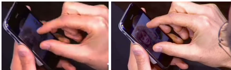
Figure 8.2: The Fingers apart gesture as it is used on the Apple iPhone for resizing images.
