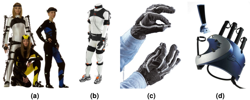
Figure 2.6: Examples of wearable sensors for arm's length and distal scale interactions. (a) Animazoo's 4 Gypsy 6; (b) XSens's 5 MVN; (c) The Fakespace 6 Pinch glove; (d) The Inition 7 P5 glove.
